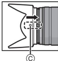
2 Turn the lens hood in the direction of the arrow until it stops, and align the stop mark **D** on the long side of the lens hood with the mark on the tip of the lens.
