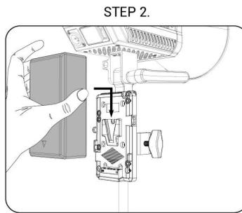
Mount the V-mount battery onto the plate.
