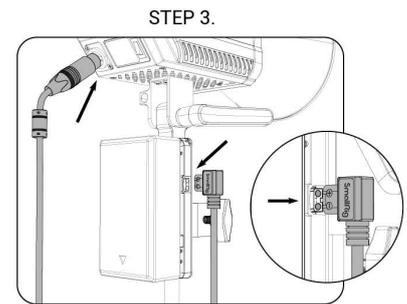
Connect the light with the battery through the D-tap cable.
