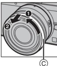
**1** Rotate the decoration ring **(C)** in the direction of the arrow to remove it.
